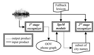
Figure 1. Overview of proposed the two-stage recognition system.
